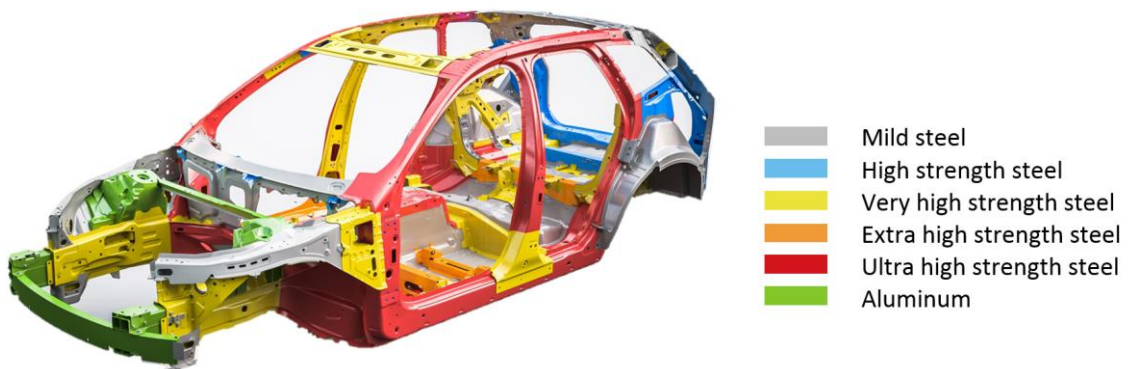
Figure II. 30 Volvo XC60 body structure [Volvo, 2017].
