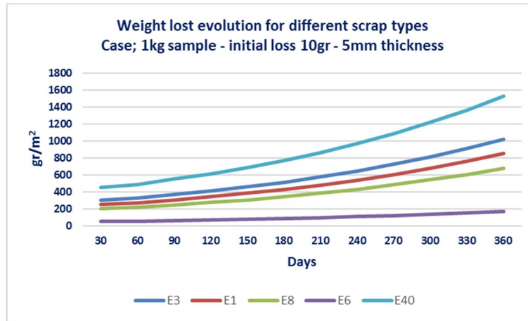
Fig. 7.45: Weight lost evolution for different scrap materials according initial material characterization data for the selected example
