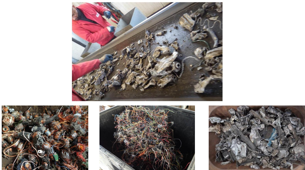
Fig. 5.3: Up) Hand picking after shredding. Down) No-Ferrous material sorted from the scrap stream
