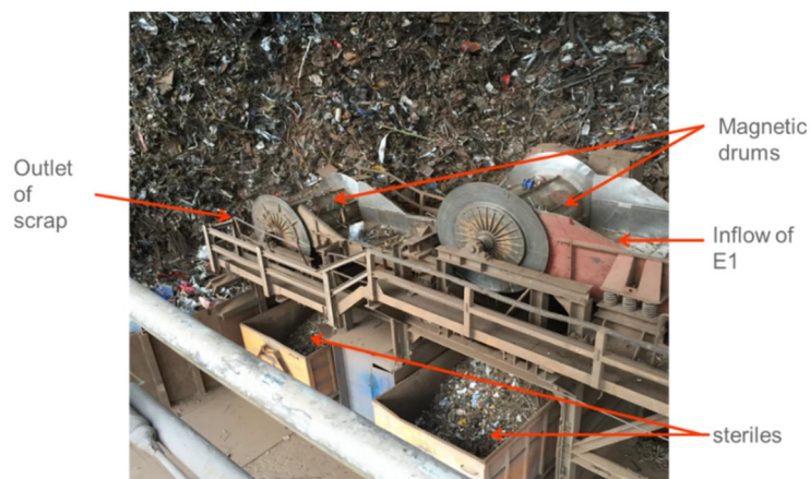
Fig. 6.6: Scrap cleaning machine description
