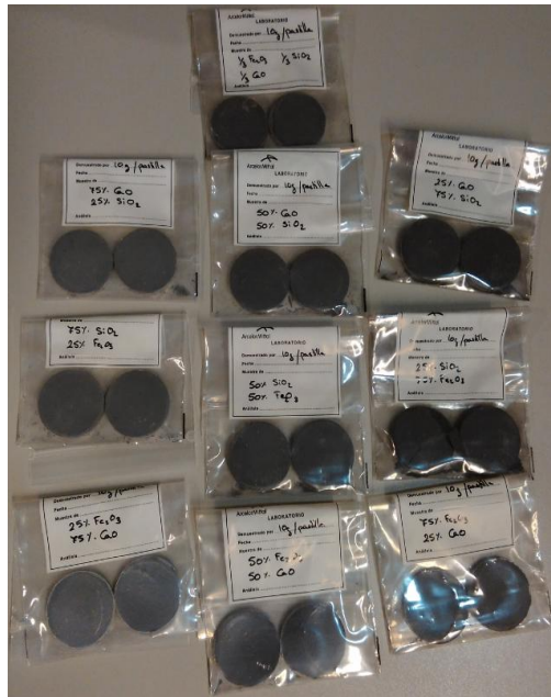
Fig. 8.59: Chemical composition of Mixed compounds pellets
