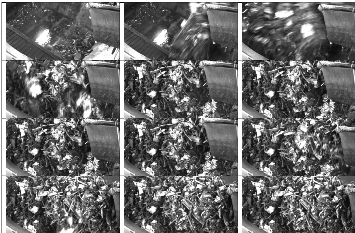
Fig. 9.66 :Scrap discharging sequence acquired at 638 nm
