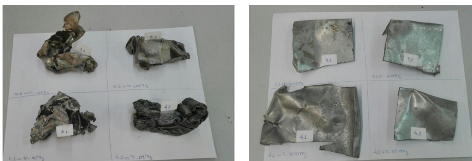
Fig. 7.23: Appearance of samples after pickling
