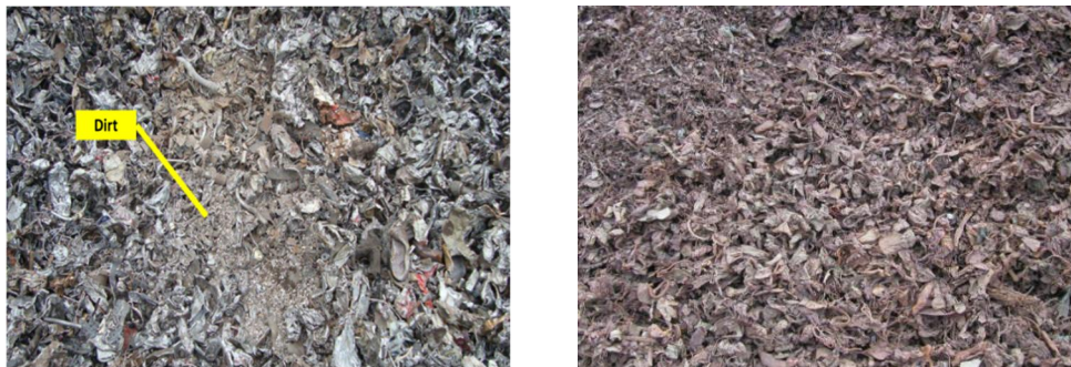
Fig. 4.2: Example of higher amount of dirt than allowed (left) and highly oxidized scrap (right)
