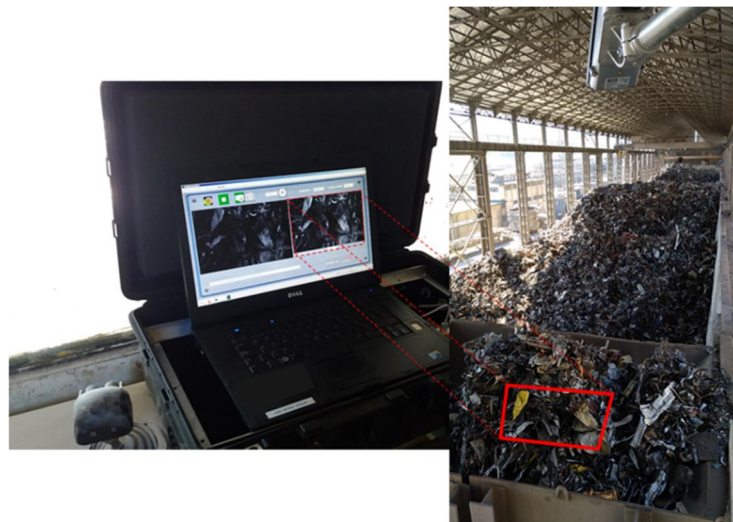
Fig. 9.64: Region of Interest (ROI) of camera over the cleaning machine feeding conveyor
