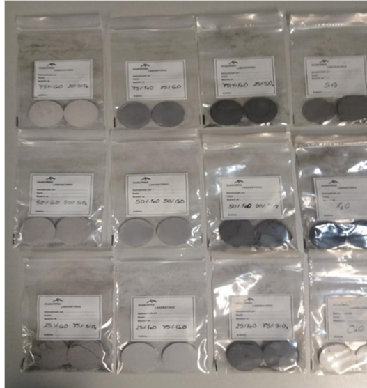
Fig. 8.80: Pressed pellet of pure compound mix to simulate scrap sterile
