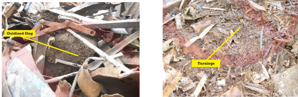
Fig. 4.4: Example of higher amount of dirt than allowed (left) and scrap grades mixing (right)
