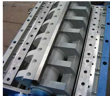
Fig. 5.15: left) rotor of a blades mill. right) fixed blades situated in the rotor of a blade mill
