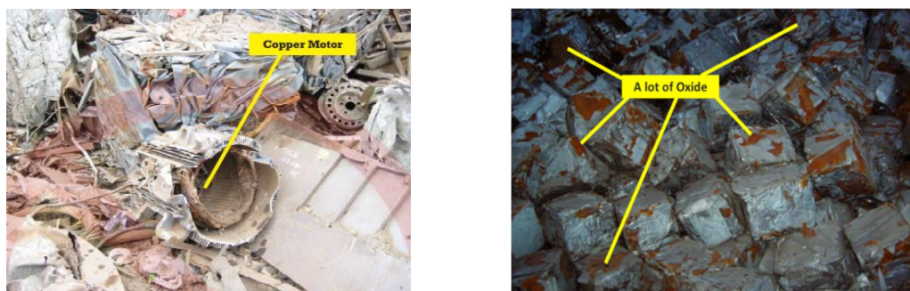
Fig. 4.8: Example of non-allowed elements in E6 scrap (left) and Highly oxidized scrap (right)
