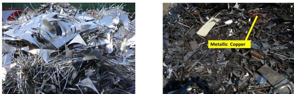
Fig. 4.10: Example of tin coated busheling (left) and (right)
