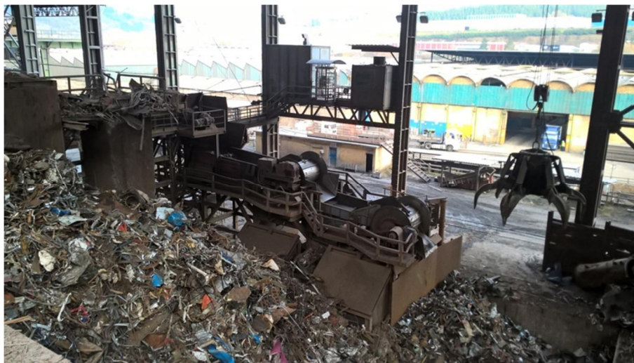
Fig. 9.2: E1 Scrap cleaning machine at one ArcelorMittal site in Spain
