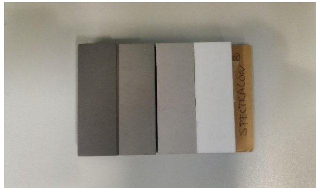
Fig. 8.76: Spectralon based calibration plate
