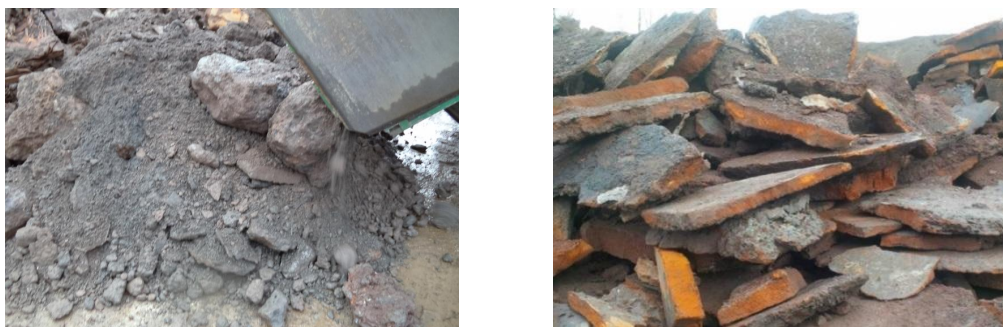
Fig. 4.12: Example of high slag content (left) and (right) big pieces of BI
