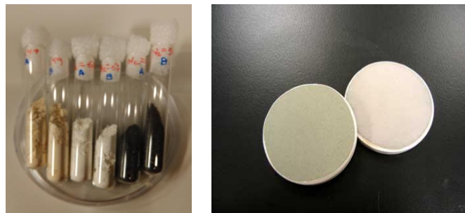
Fig. 8.25: Samples of sterile to be analyzed: Left) pipette and Right) pressed pellet
