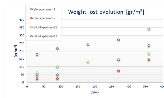
Fig. 7.41: Weight lost evolution for all analyzed samples
