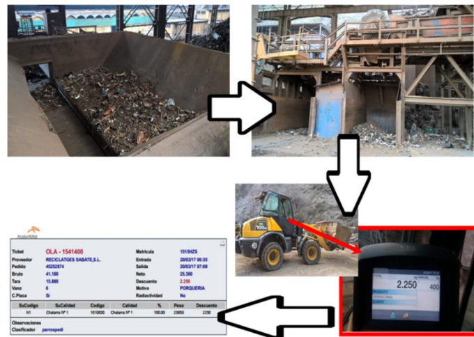
Fig. 6.7: Sterile weight characterization at the scrap cleaning machine
