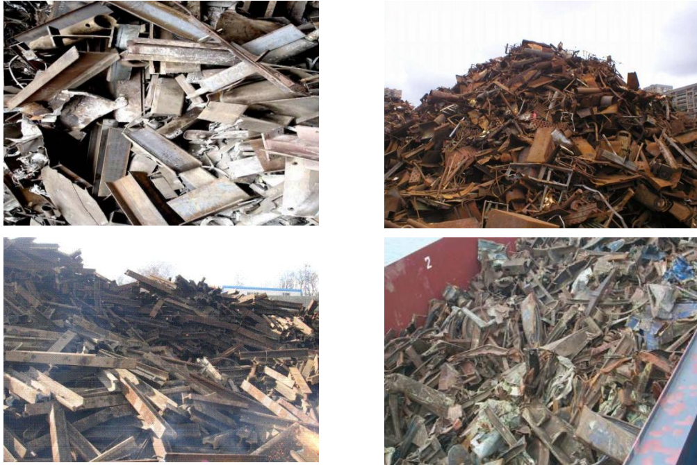
Fig. 4.5: E3 scrap examples: Top-left) USA, top-right) Spain, bottom-left) rail and bottom-right) Belgium
