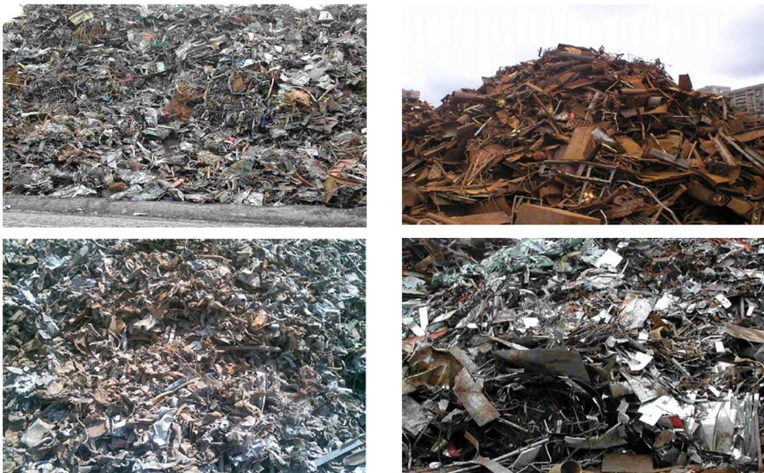
Fig. 9.14: Examples of Scrap types: Up left) Old Light scrap, Up right) Old heavy scrap, Down left) Old fragmented scrap, Down right) New production thin scrap
