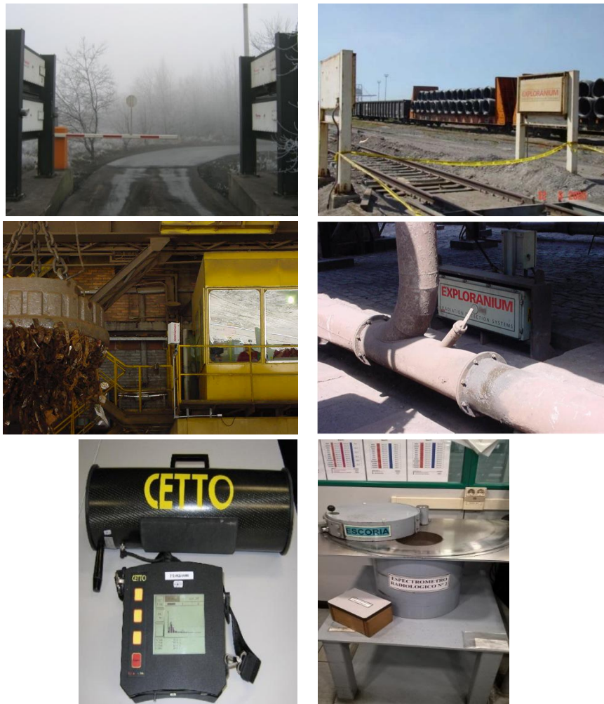
Fig. 6.18: Different radioactive controls: Up) Portal control for Scrap delivery by truck and by train, mid) Scrap and dust on line control and Down) punctual analyses
