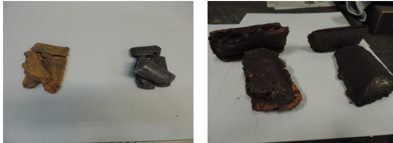
Fig. 7.5: HBI specimen with different atmospheric exposure times
