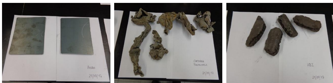
Fig. 7.9: Selected specimens. Left) Busheling scrap (E8), middle) Shredder scrap (E40) and right) HBI samples
