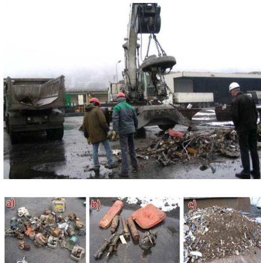
Fig. 6.5: Up) Quality control on concrete area. Down) Elements containing Cu (a), sealed elements that can explode in the furnace (b) and sterile remaining on the floor (c)
