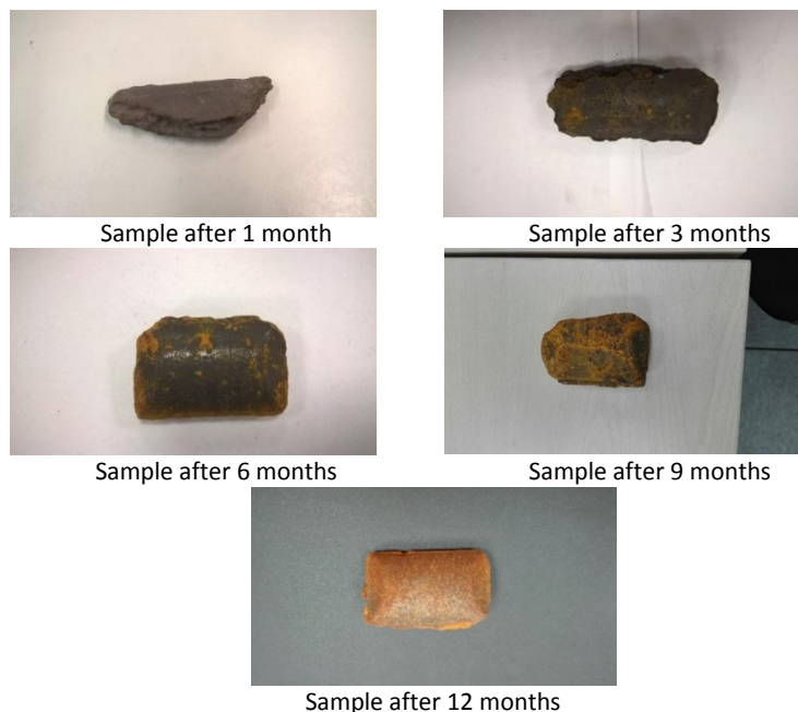
Fig. 7.16: Visual appearance after different exposure periods of samples in experiment 1
