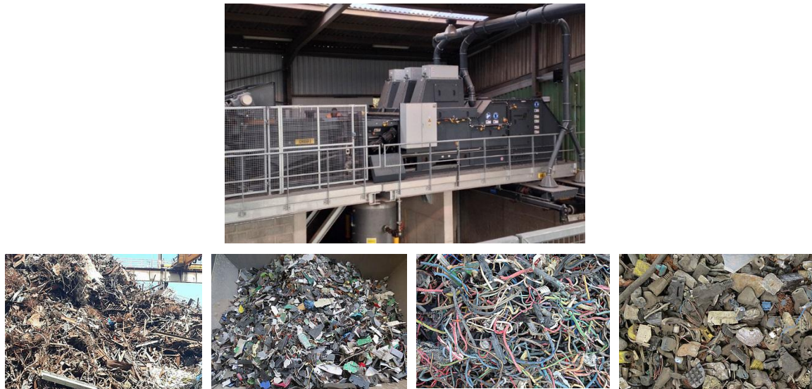
Fig. 5.35: Up) Color separation technology (51). Down) Different materials to treatment, from left to right: sheared scrap, electronic scrap, wire processing, shredder residue.
