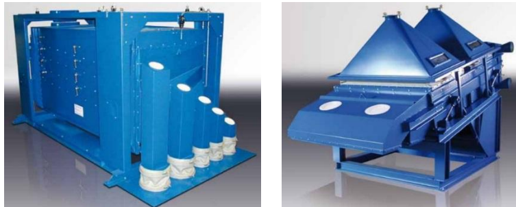
Fig. 5.20: Example of industrial screen for separating by sizes during metal waste processing (32)
