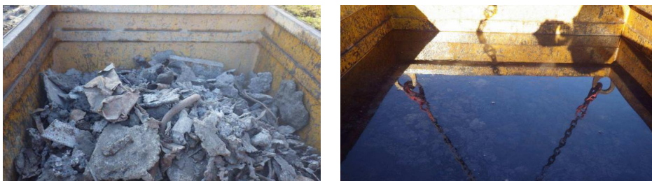
Fig. 6.15: Water displacement method
