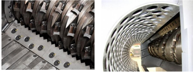
Fig. 5.16: Left) Detail of a blades crusher. Right) Blade crusher with perforated grill
