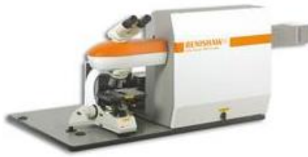
Fig. 8.22: InVia Raman Spectrometer technical characteristics
