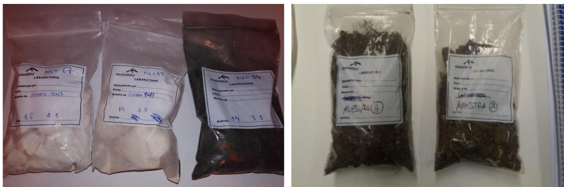
Fig. 8.27: Raw material used for experimental tests; Left) Pure compounds (Lime, Dolomite and SiO 2 and Right) real sterile
