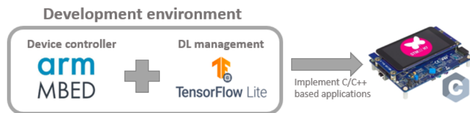
Figure 4. General structure of the development environment used for deep learning (DL) integration into embedded systems.
