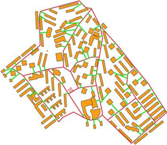
Figure 3. District heating network proposal main loop (red) with building interphase connections (green)
