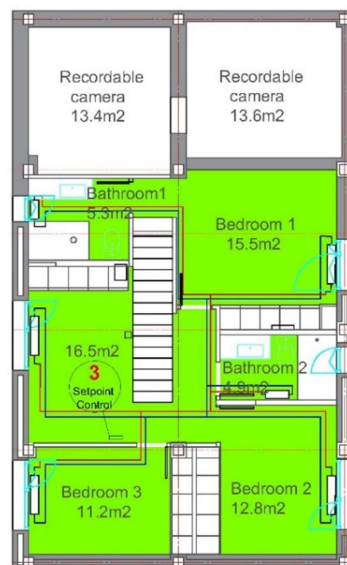
Figure 9. Scheme of installation heating system with zonal control(Z3); 1: setpoint control in Txoko (1st floor); 2: setpoint control in living room (2nd floor); 3: setpoint control in corridor (3rd floor). Three types of color indicate the heated areas for each floor.
