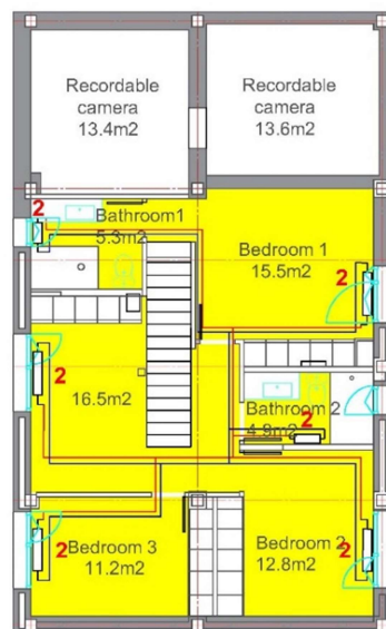
Figure 8. Scheme of installation heating system with zonal control; (1: boiler; 2: terminal units; 3: setpoint control: 3 a - setpoint control in the living room (Z1), 3b-Setpoint control in the kitchen (Z2)). Yellow color indicates the heated areas.
