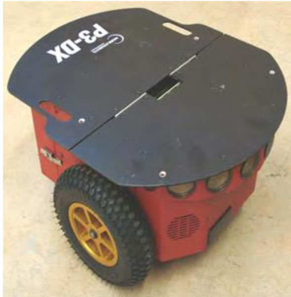
Figura 29: AGV Pioneer 3 original
