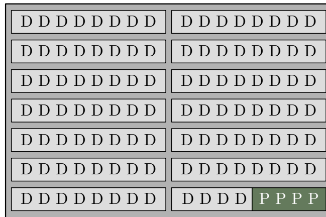
Figure 4.5: Padding applied to an unaligned input data. Data is represented by 'D' and padding by 'P'.
