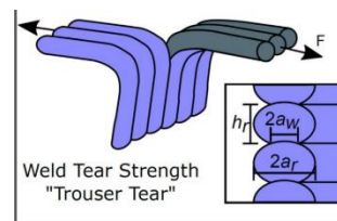
Figure 17: Trouser-test specimen tear direction. Adapted from reference (34).
