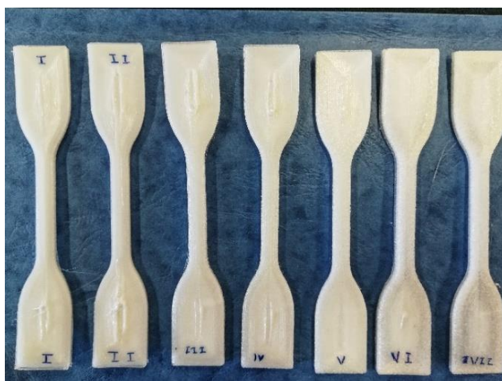
Figure 38: Tensile-test printed specimens of seven different printing conditions with the concentric filling pattern.
