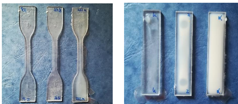
Figure 19: Injected specimens at three different mould temperatures. From left to right the mould temperature increases. (25, 70 and 85 °C).
