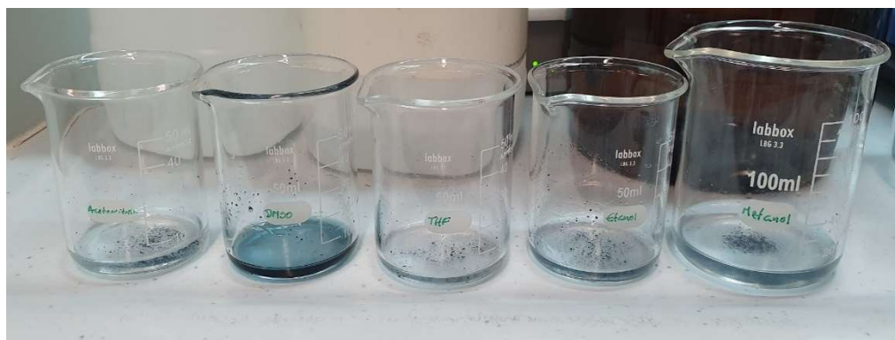
Figure 18 - Solubility test for PEDOT:PDADMA-AQ. From left to right, Acetonitrile, DMSO, THF, Ethanol, Methanol.
