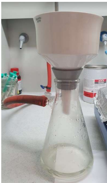
Figure 6 – Arrangement used to perform a vacuum filtration.
