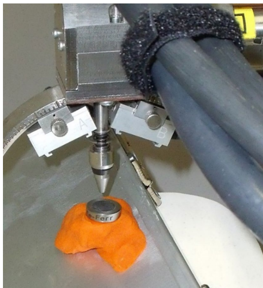
Fig. 9 Detail of the calibration process on a powder sample. The “A” and “B” radiation detectors identify the angle of the diffracted radiation ( 2\theta_0 )
