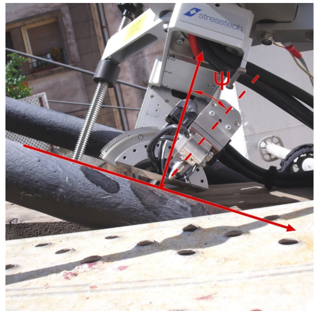
Fig. 5 Position of the X-ray emitter in the goniometer scanning process (circular element in the image). Its inclined position is observed perpendicular to the bar
