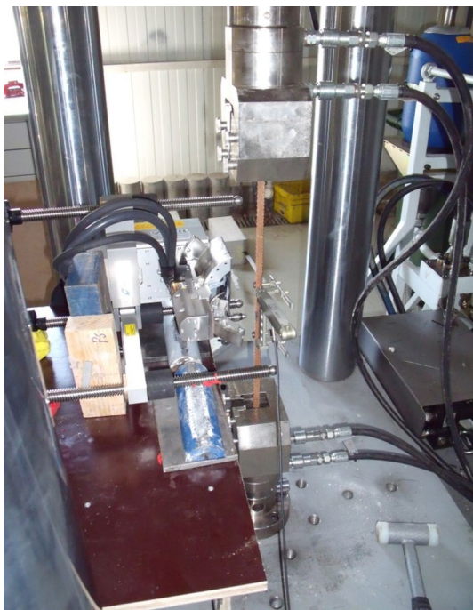
Fig. 12 Positioning of the diffraction equipment before starting the calibration process
