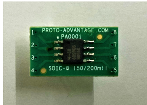
Figure 14: MLX90395 chip soldered into a DIP-8 SMT Adapter.
