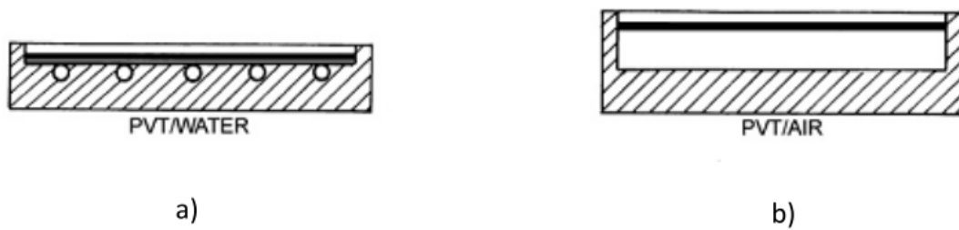
Figure 22. Diagram of a cross section of a) water-cooled PVT collector; b) air-cooled PVT collector (Kalogirou, 2015).
