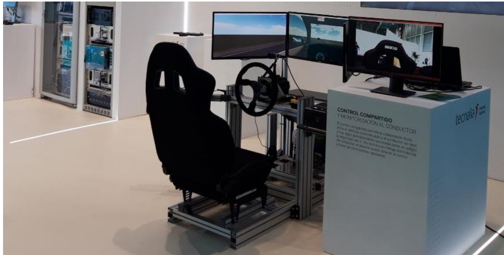
Fig. 3.3: Driver-in-the-loop AD simulator platform of Tecnalia
