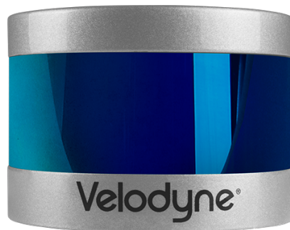
Figura 1.5: LiDAR Velodyne Puck.
