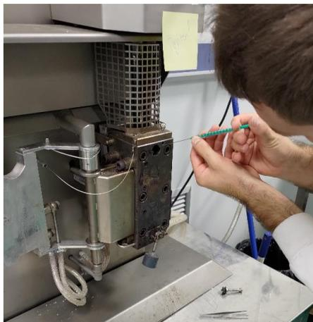
Figure 6 : Injection of PEG in the DSM
