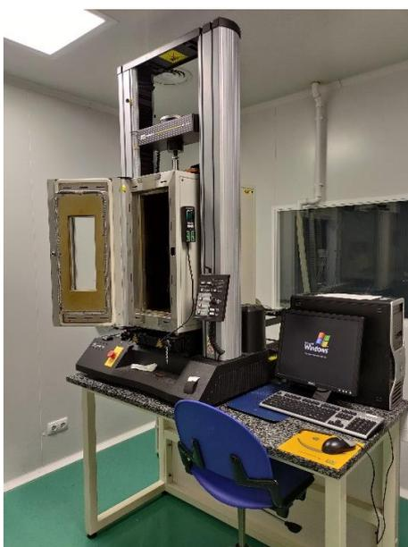
Figure 7 : Tensile test machine and control box
