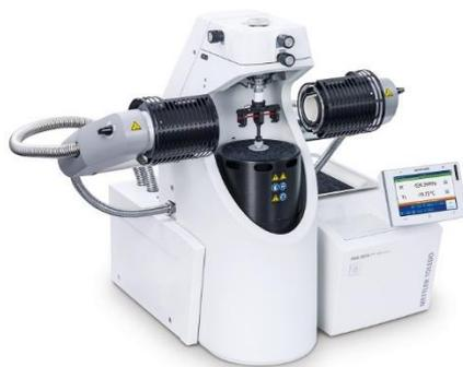
Figure 10 : DMTA Mettler Toledo
