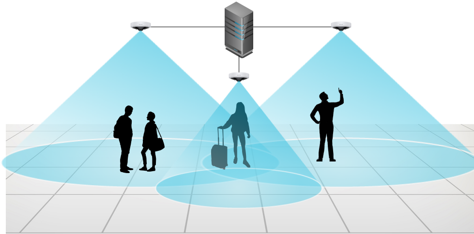
Fig. 2.8: Illustration of the considered scenario. Multiple omnidirectional cameras with a small overlap cover the monitored area. The cameras are connected to a central GPU-enabled server.
