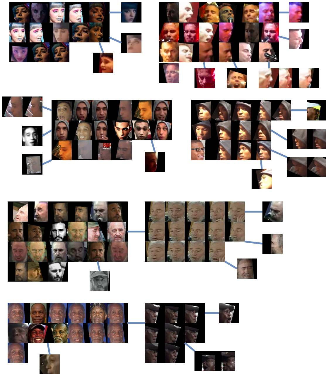
Fig. 11. Example clusters and connections generated by the proposed method in the IJB-C + 3 millions of distractors from VGG2 experiment. Each group of contiguous faces represents a cluster and each line represents a connection.
