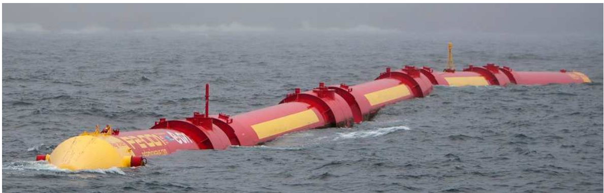
Figure 7.7: Pelamis P2 device, pictured at the European Marine Energy Centre, 2011.
