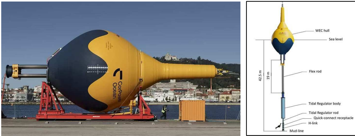
Figure 7.13: CorPower C4 hull (left) and schematic (right).
