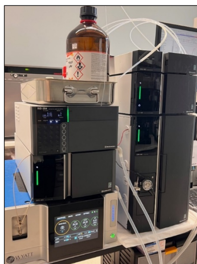
Figure 10: Shimadzu Nexera 40 HPLC system employed in this work.
