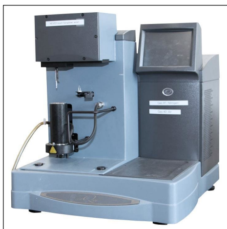
Figure 9: Q500 TA INSTRUMENTS equipment for thermogravimetric analysis.
