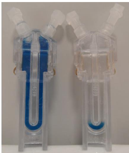
Figure A. 10. -A. Cell entirely filled with blue dextran in 10 mM NaCl. B. Cell filled with 10 mM NaCl and loaded with 50 \mu\text{l} blue dextran for the diffusion barrier 14 .
