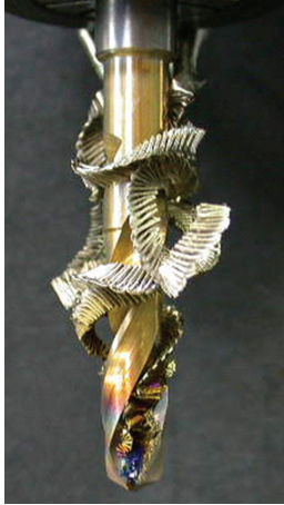
FIGURE 6: Tool blocking caused by the accumulation of material in the chip flow zone.
