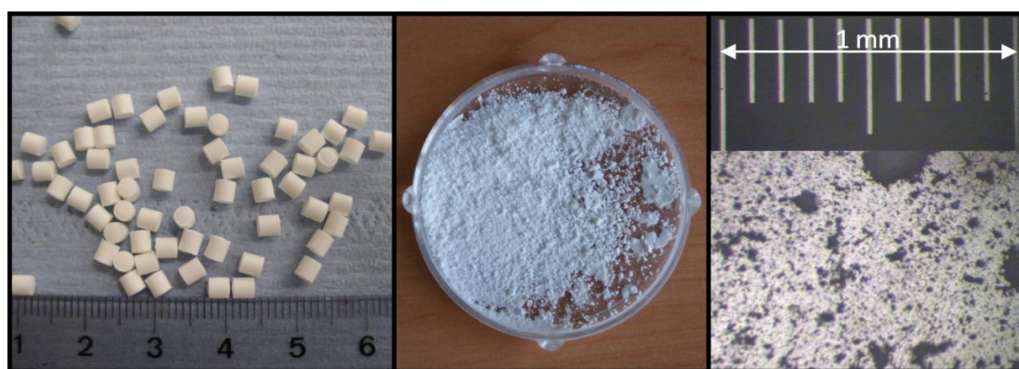
Figure 6.20 Appearance of alumina pellets before and after the experiment. The last picture shows the appearance of \text{Al}_2\text{O}_3 pellets after the experiment and it was taken with an optical microscope.
