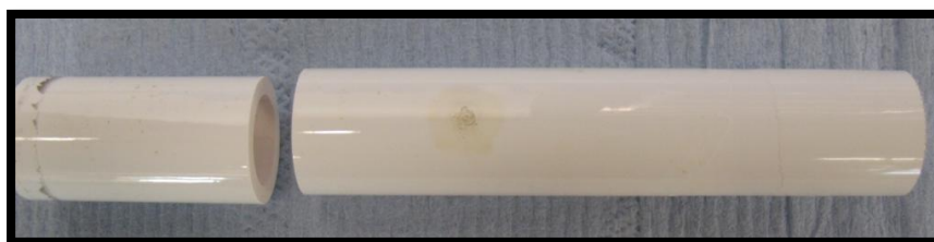
Figure 6.21 Physical appearance of the membrane after performing the experiment with Amberlyst resins and alumina particles.
